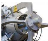
The separator has an air driven head with four separate moving valves that provide a great deal of counter pressure. Therefore it can separate even the thinnest manure/digestate/sludge without any risks.
