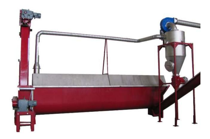
**Function:** To cool down hot product directly from the cooker section or press section. The product is cooled by counter-flow air which is drawn through the cooling bin.
