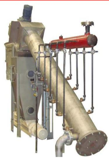
**Function:** To coagulate continuously the raw blood flow with injected direct steam into a blood clot which is ready for further processing/drying.
