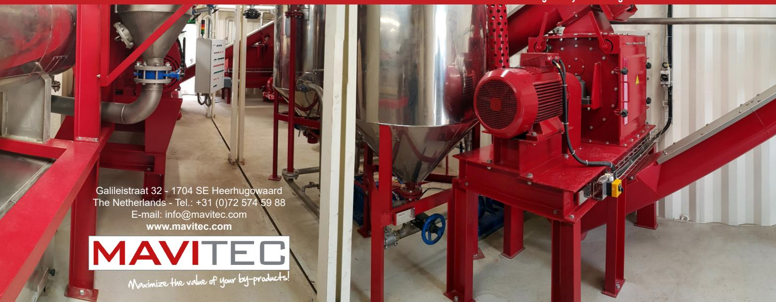
The **containerized batch solution** is a fully functional rendering plant designed to process small quantities of poultry or red meat by-products. With it's small footprint this unit is suitable to be placed inside a small building or even outside if the weather conditions allow it. The container is based on a 'plug and play' system: it just needs to be connected to the water, steam and electricity supply. If equipped with defatting container the containers need to be connected.
