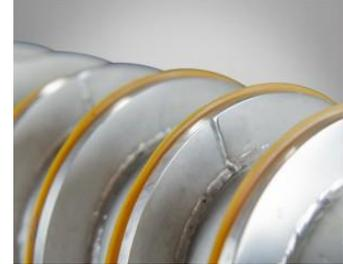
The auger in this separator has bearings on both sides. Because of this the auger is always positioned in the centre of the machine. This prevents unnecessary wear.
