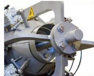
The separator has an air driven head with four separate moving valves that provide a great deal of counter pressure. Therefore it can separate even the thinnest manure/digestate/sludge without any risks.
