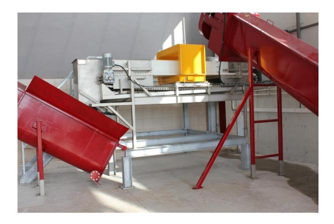
**Function:** To detect and separate any metal pieces from your raw product before entering the production process
